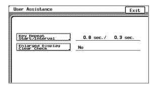
Touch and all to specify the desired length of time until the repeat feature for a key starts (between 0.1 and 3.0 seconds).
